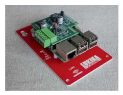
RS232 serial connection to the control panel with a terminal block.
